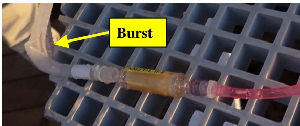
Fig. 3-3-4. Burst tube (left) and clogged filter (right)
