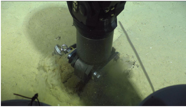
Sediment sampling using M-type corer
