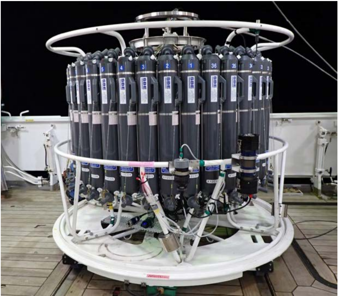
Fig. 3-3-2. MASS Pump installed on a CTD water sampling system
