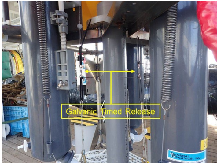
Fig.9 Galvanic Timed Release set in a Niskin water sample.
