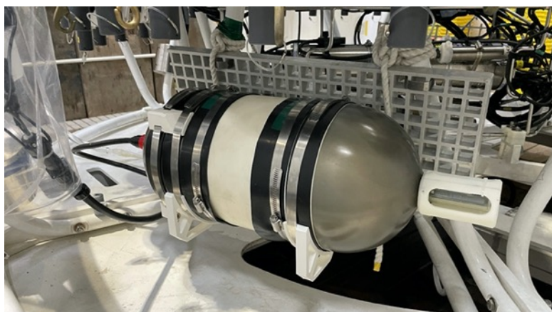
Fig. 3.2.3.1 Absolute salinity sensor attached to the CTD frame.
