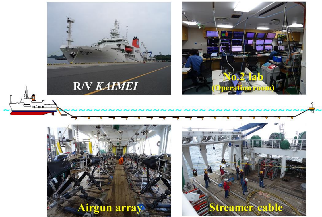
Fig. 2 Seismic system on R/V KAIMEI .
