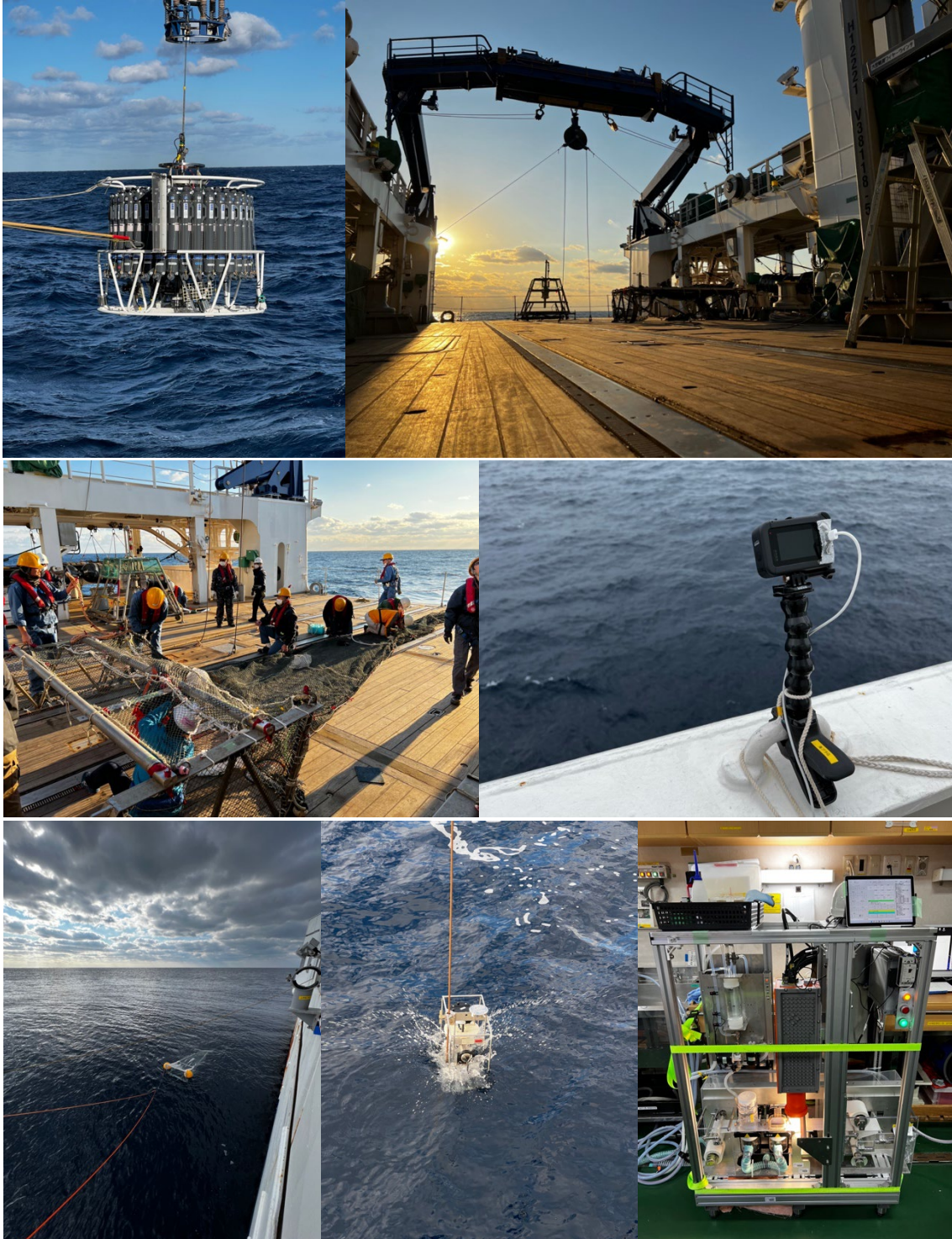
Figure 2. Survey items. CTD/Niskin (upper left), multiple corer and beam trawl (upper right), beam trawl (middle left), GoPro camera (middle right), neuston net (lower left), in situ pump (lower middle) and microplastics detection system with hyperspectral camera (lower right)
