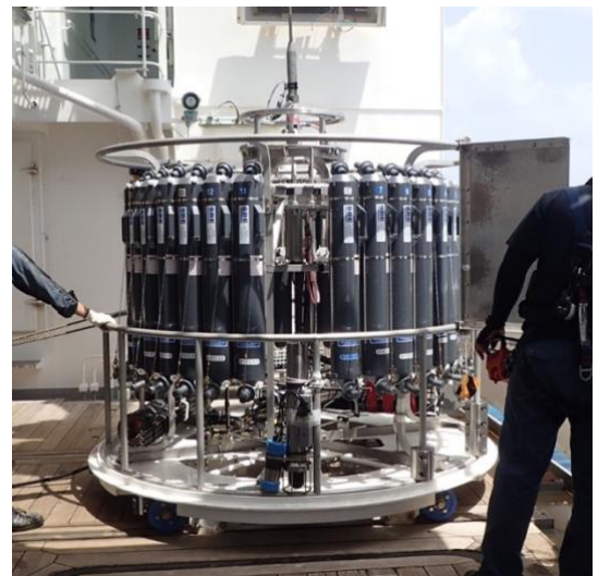
Fig. 3-3-4 CTD system with LADCP, LISST, shadowgraph camera
