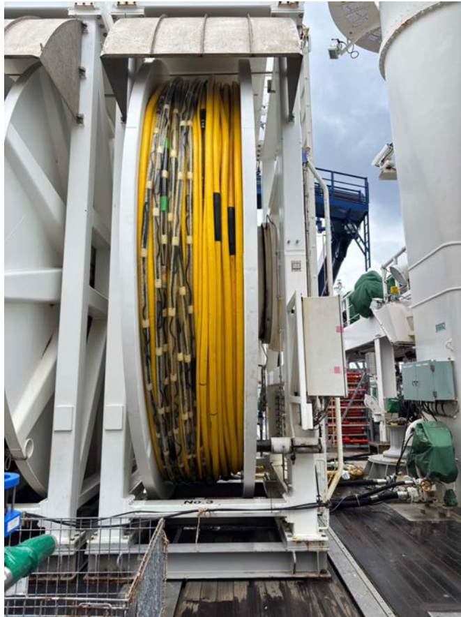
Figure 5 Multi-channel hydrophone streamer cables.
