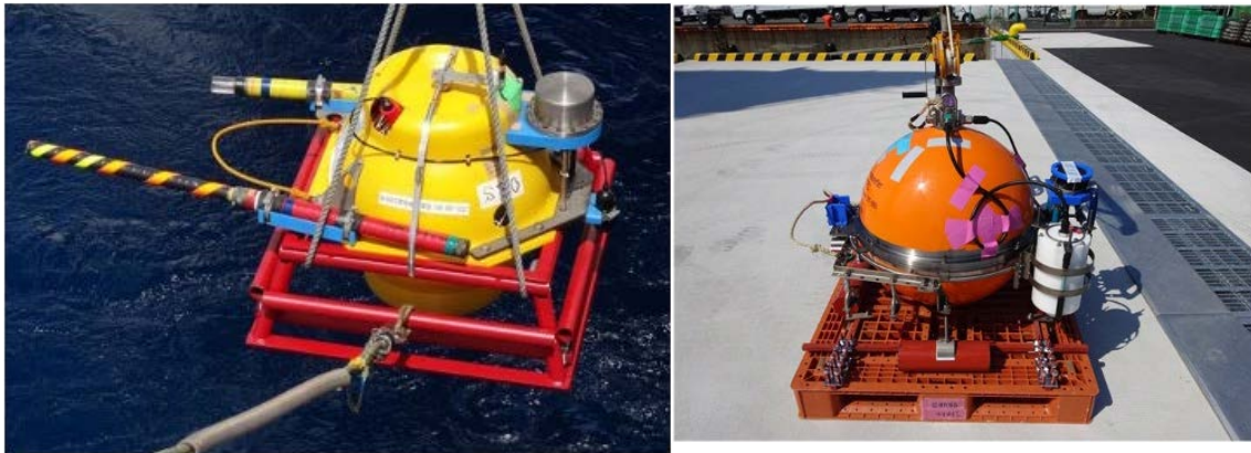
Figure 7 External views of the OBSs used for long-term seismic observation. SPOBS (left) and BBOBS (right).
