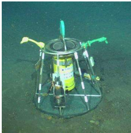
Fig.4-2-10-3 ADCP installed at the lander site (Stn. HG_LS)
