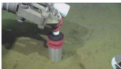
Sediment core sampling
