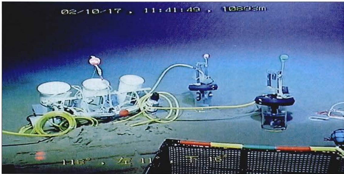
Figure 1. Benthic respirometer deployed on the seafloor at 10, 893 m.
