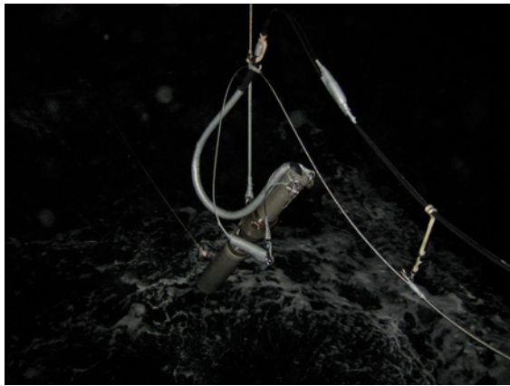
Fig. T. Tangled retrieval wire and towing harness (left) and chafe-protected stainless steel snap shackle (right).
