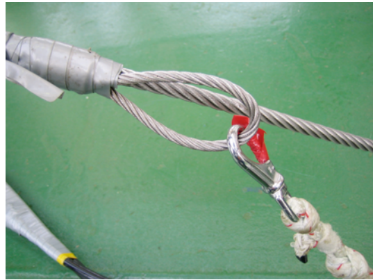
Fig. T. Tangled retrieval wire and towing harness (left) and chafe-protected stainless steel snap shackle (right).
