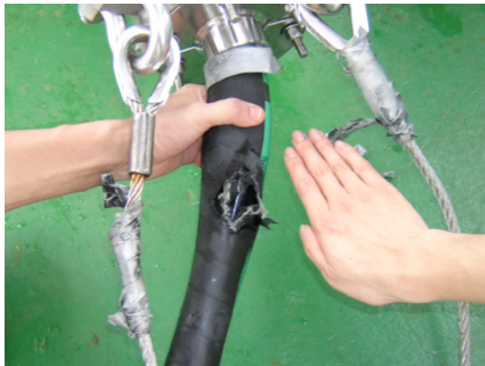
Fig. S. Ruptured protective air hose and firing line sheath.
