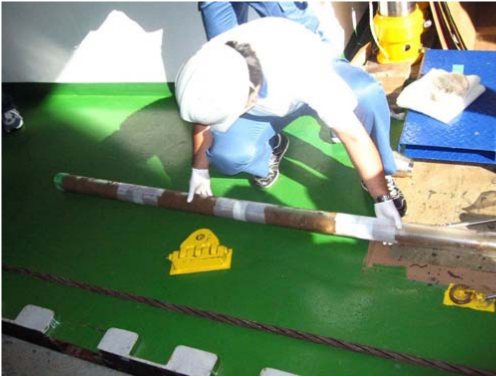
A mud sample (length = 1600 mm) was taken from the sea bottom in the depth of 10,350m
