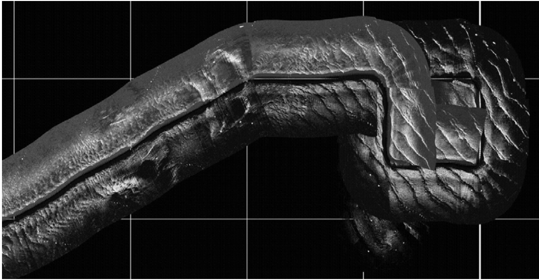
Fig.3-7-2 A close up map of the side-scan backscatter mosaic map during the No. 43 rd dive of r2D4 with a resolution of 1 meters . (about 4200m×2000m)
