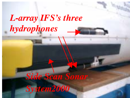
Fig.3-2-5-2 Photo of the L-array interferometry sonar system
