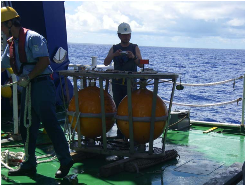
Figure 4. Two lithium battery frames recovered from the WP-1 sea floor borehole seismic observatory at the site 2 by two KAIKO-7000II dives (#455 and #456).
