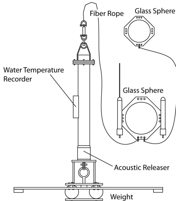
Figure 3.4-4. Schematic drawing of PWT.
