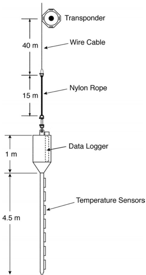
Figure 3.4-3. Configuration of the heat flow measurement system using a deep-sea probe.
