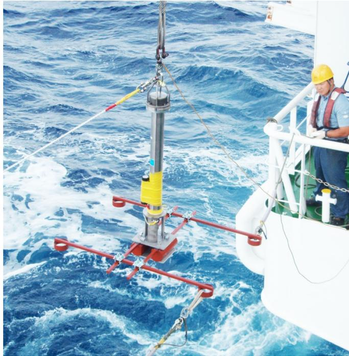
Figure 3.5-2. Deployment of a pop-up water temperature measurement system (PWT).
