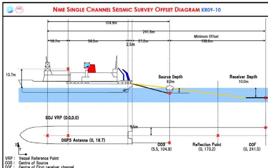
Figure 3.4-1: Schematic figure of SCS towing system
