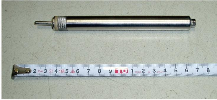
Figure 3.4-2. ANTARES Miniaturized Temperature Data Logger (MTL).
