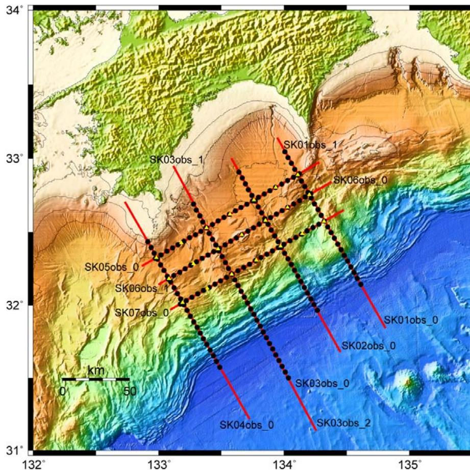
Black circles and yellow triangles show locations of deployed OBSs for a long-term observation and them for short-term observation, respectively. Red lines are seismic refraction/reflection survey lines conducted in this cruise using a tuned air-gun array and OBSs.
