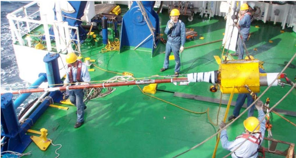
Figure 3.4-1. Deep-sea heat flow probe.
