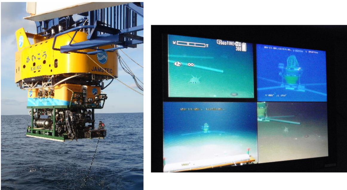
Figure 3.5-17. Left: ROV Kaiko recovered from the CSEM experiment. The 20m-dipole cable can be seen, extended from sample basket. Right: OBEM taken by ROV Kaiko Camera at site A5.
