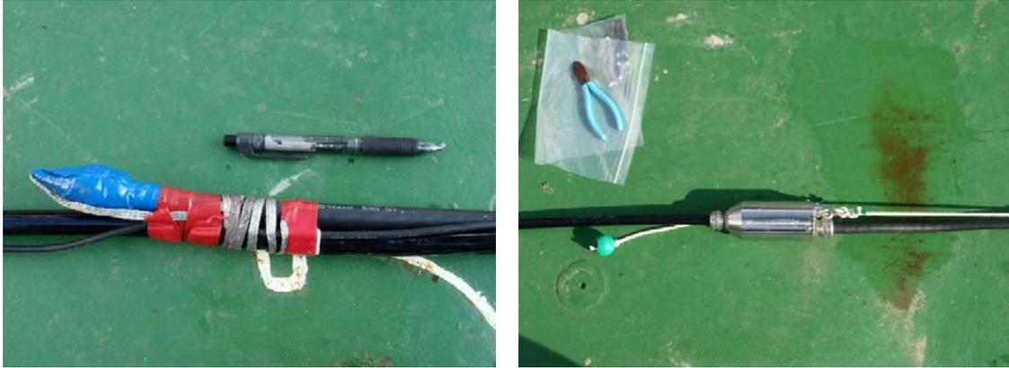
Figure 3.4-20. Source Electrode (left) and cable termination (right).
