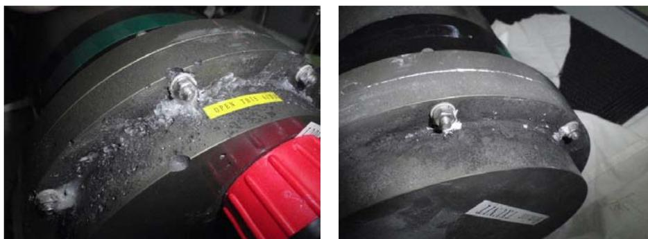
Figure 3.5-18. Electrical corrosion by leakages at the TX unit.
