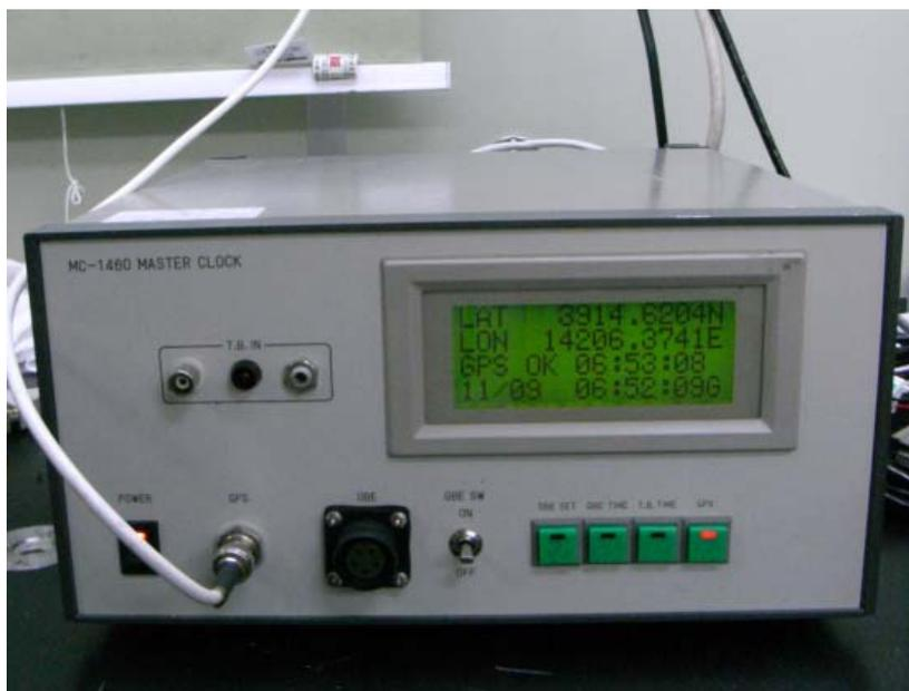
Figure 3.4-13. Photo of the developed NTP server unit.
