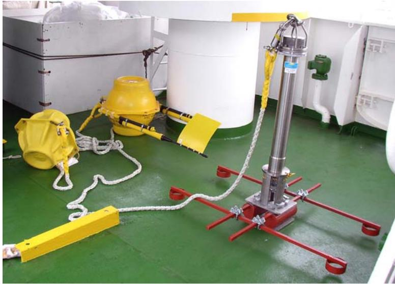
Figure. 3.4-9. Pop-up water temperature measurement system (PWT).
