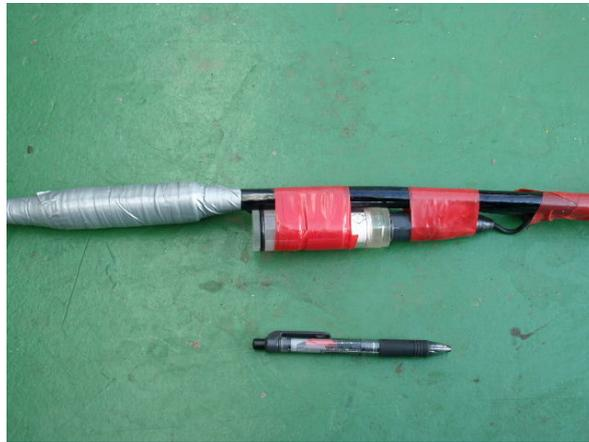
Figure 3.4-21. Receiver electrode (Ag-AgCl).
