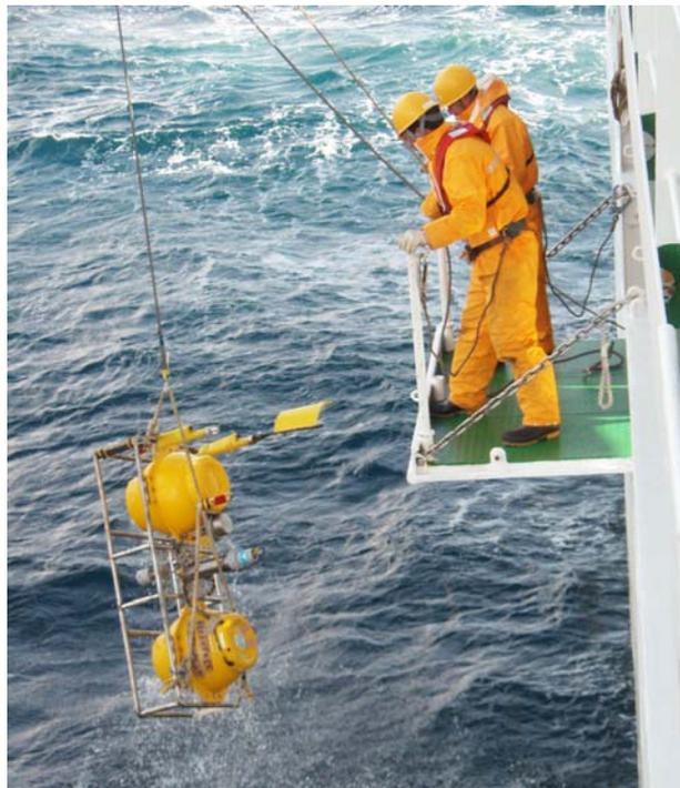
Figure 3.5-1. Recovery of a pop-up heat flow instrument (PHF).
