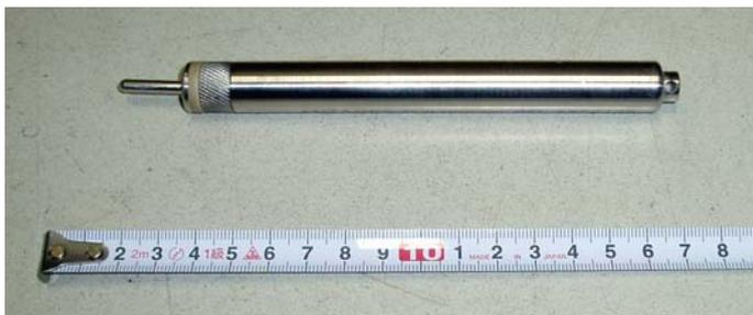
Figure 3.4-2. ANTARES Miniaturized Temperature Data Logger (MTL).
