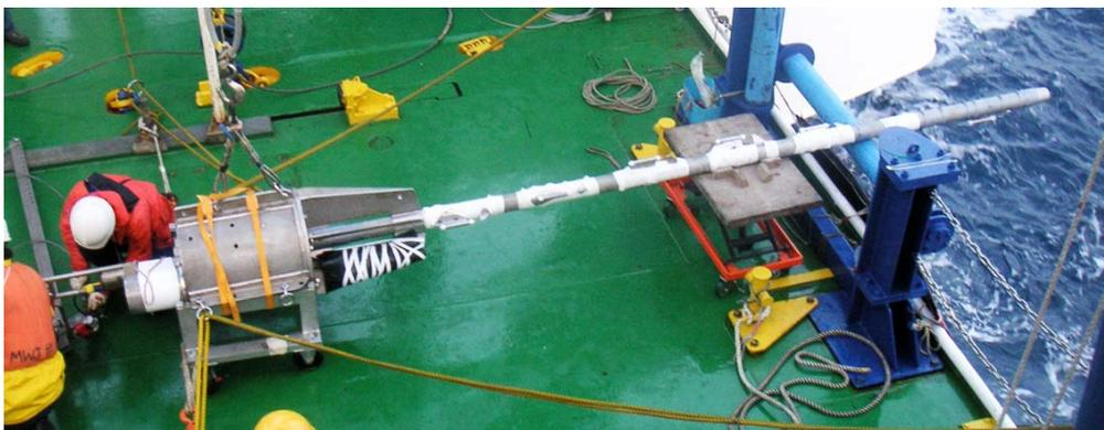
Figure 3.4-5. HFPC with compact temperature data loggers (MTLs).
