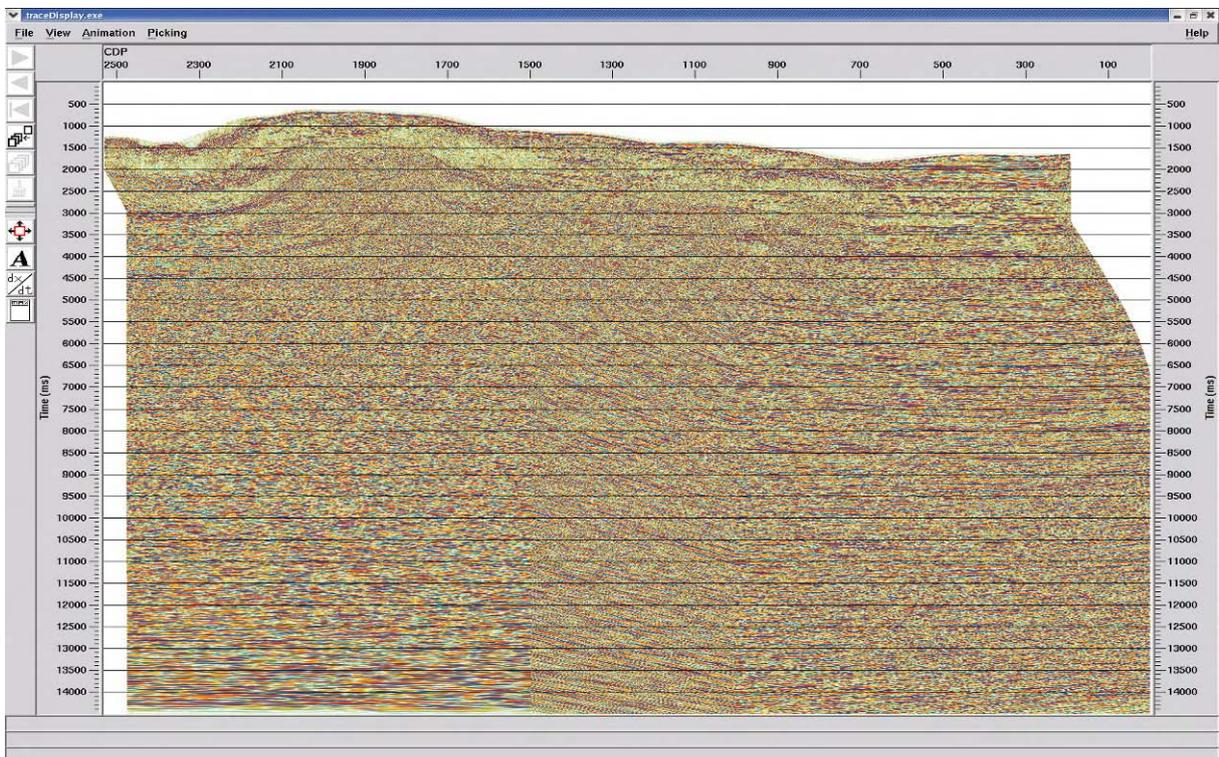
Fig.9 Example of MCS profile with onboard processing (Poststack time migration section of Line SG10-B).
