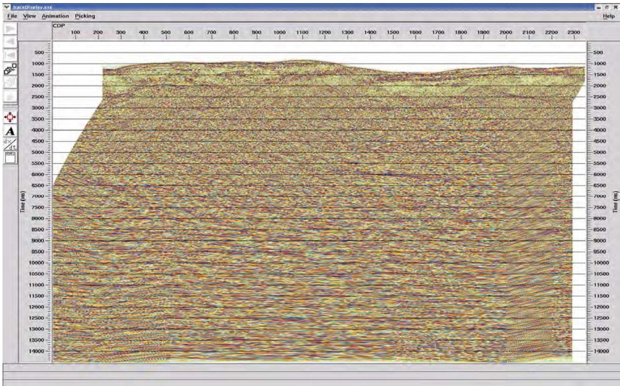
Fig.8 Example of MCS profile with onboard processing (Poststack time migration section of Line SG10-A).
