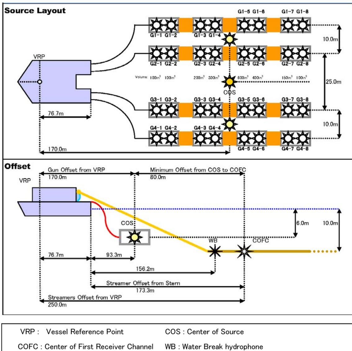
Fig.3 Example of vessel towing geometry (SG10-1, SG10-2, SG10-C, SG10-EW1, SG10-EW2, SG10-EW3, SG10-EW4). Top figure shows the source (airgun system) layout, bottom one represents source-receiver depth and position, and navigation offsets.
