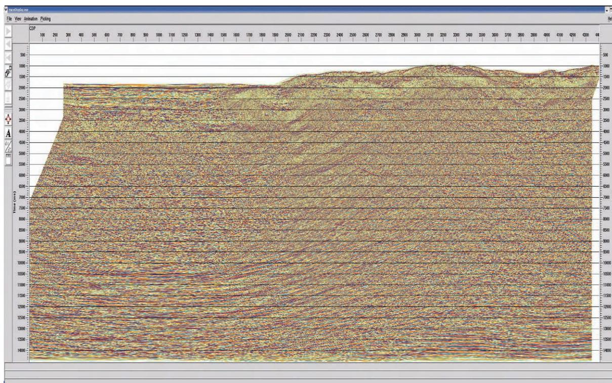
Fig.7 Example of MCS profile with onboard processing (Poststack time migration section of Line SG10-2).
