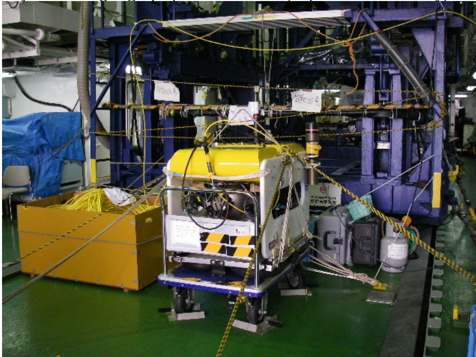
Adjustment in garage, preparation for dive (Replacement of battery).
