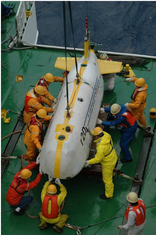
R2D4 has been laid on the carriage.
