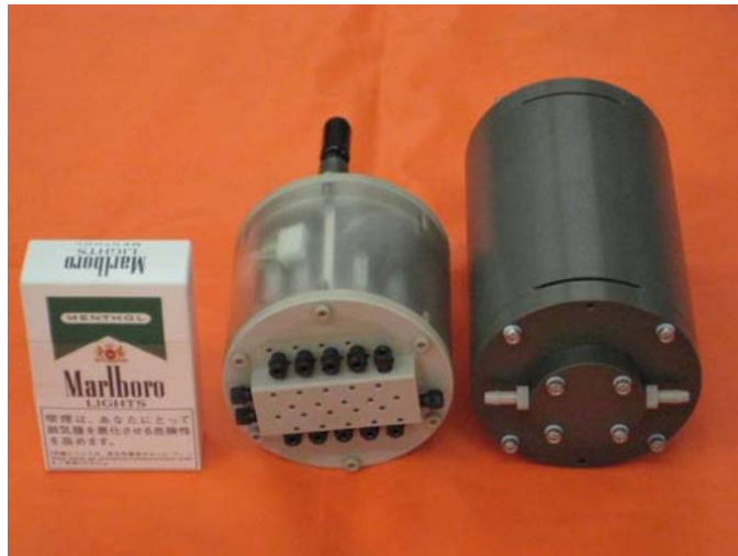
Fig. 2.3.4.1 Feature of the GAMOS (Size Comparison with a cigarette packet)
