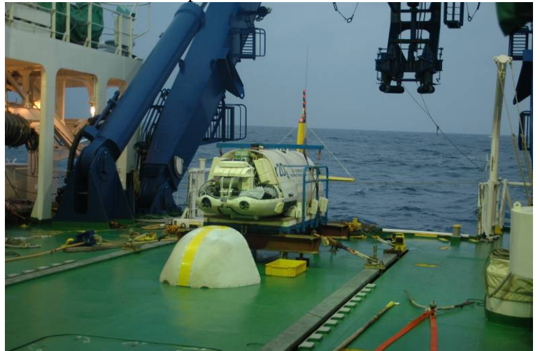
Moving to the stern on the deck, Aligning INS and Confirmed normal operation.
