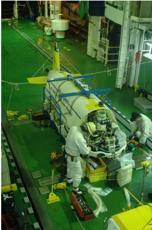
R2D4 : 4.4 m Overall length, 1.6 ton weight. Adjusting in the garage, Preparation for dive.
