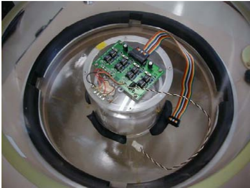
Fig. 2: OBS sensors in glass sphere
