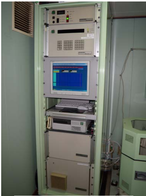
Gravity meter system rack
