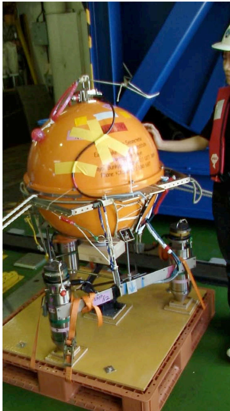
Figure 3. BBOBS-NX deployed at Site 2. The recording unit and batteries are contained in the titanium sphere (65 cm \phi ). Each of 3 component sensors are contained in the bullet shaped container held by a triangular frame.
