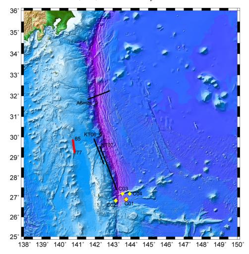
Red and yellow circles show locations of recovered and deployed OBSs, respectively. Black lines are MCS reflection survey lines conducted in this cruise using a tuned air-gun array and a 444 channel hydrophone streamer.
