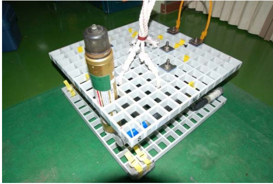
Fig.5.2.5 Photo of the “CUBE” (Compact Underwater Box-shape Electrometer). (a) Top view and (b) Side view.
