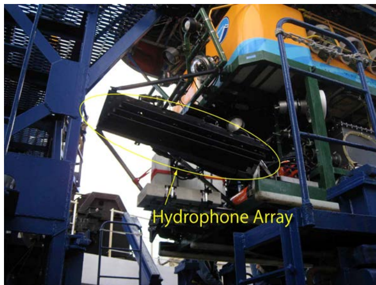
Fig5.1.2-1 Appearance of the hydrophone array of the bathymetric survey system. The length of the hydrophone array is 1.2m and forty hydrophone elements are embedded in it.
