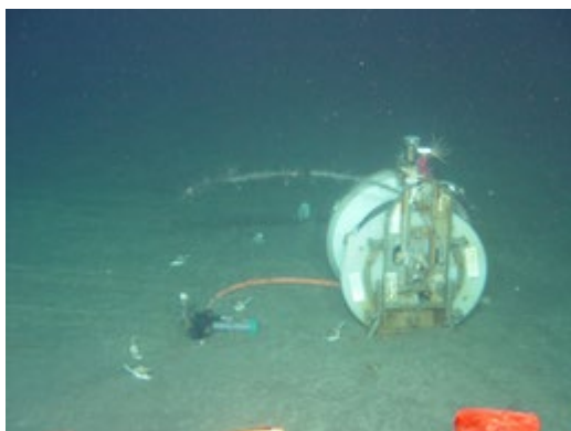
Fig.12 The Cable-Bobbin and Wet-mate Connector
