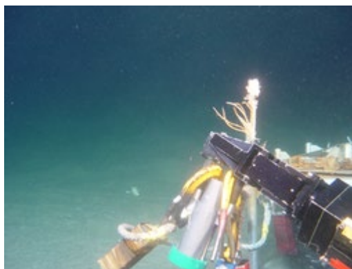
Fig.13 The Wet-mate Connector with Hooks for Recovering
