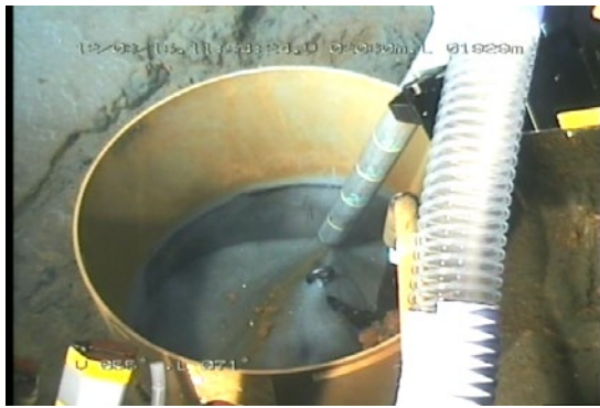
Fig.4 The removing glass beads by the DOROTHY
