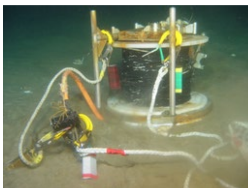
Fig.14 The Cable-Bobbin and the Wet-mate Connector with Hooks for Recovering
