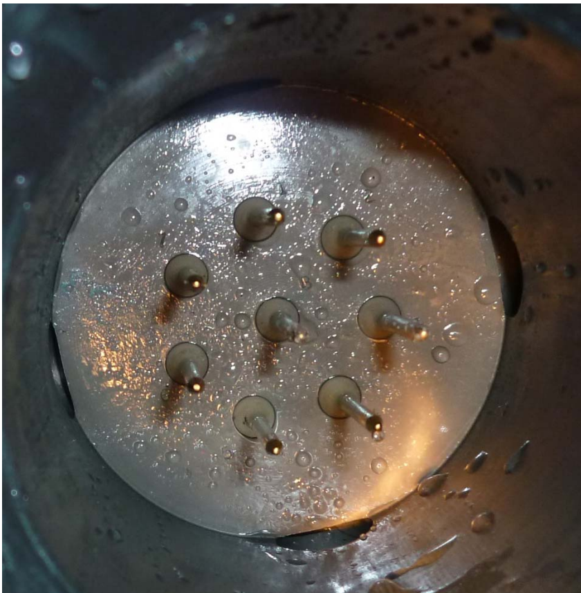
Connector pin of the SEACON ROV connector examined after dive 583.
