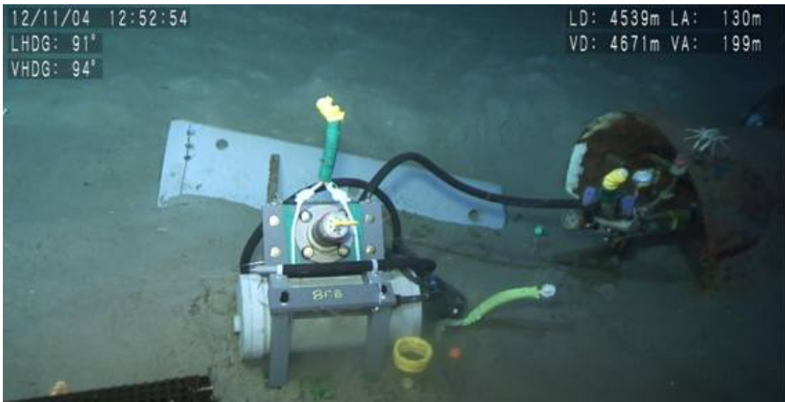
Photo of the new data logger at 808I.
