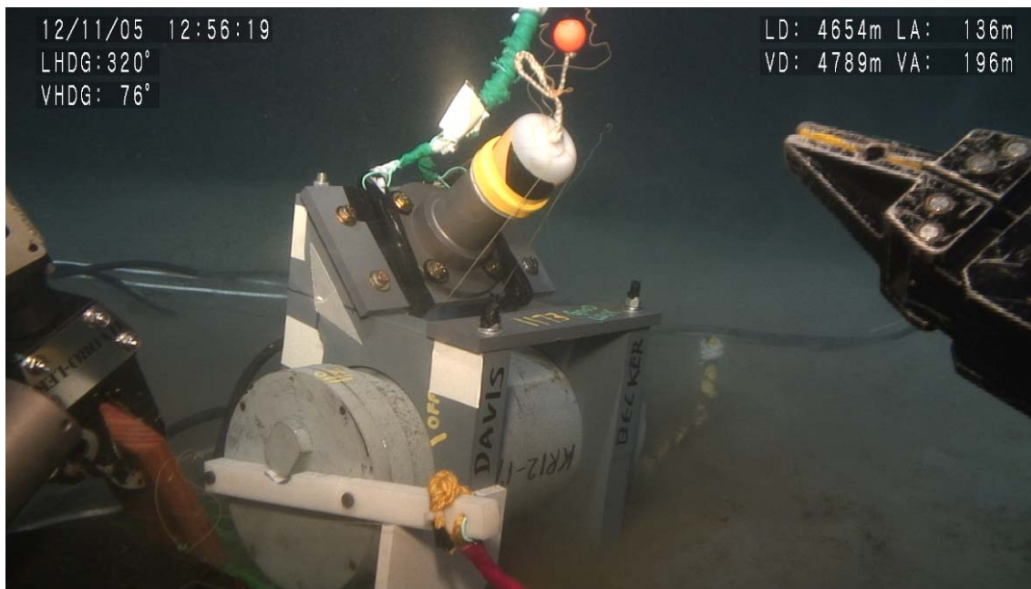
Installation of the Extension Module during dive 583. 5: Mercury switch is now ON.
