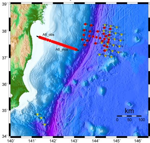
Red circles and yellow triangles show locations of deployed and recovered OBSs in this cruise and deployed them for long-term observation, respectively. Black line is seismic refraction/reflection survey line conducted in this cruise using a tuned air-gun array and OBSs.
