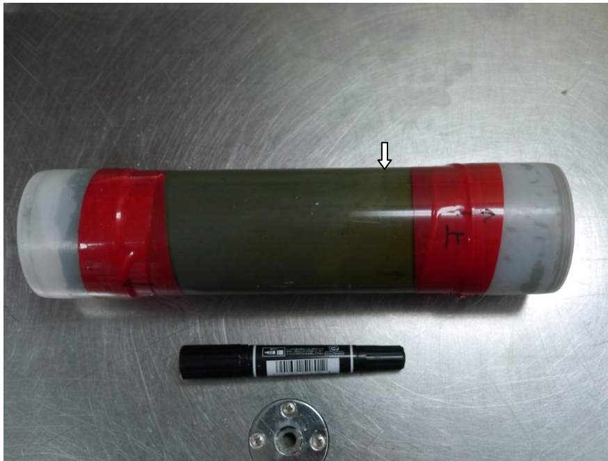
Fig. 6: Collected core sample The arrow points to the boundary.
