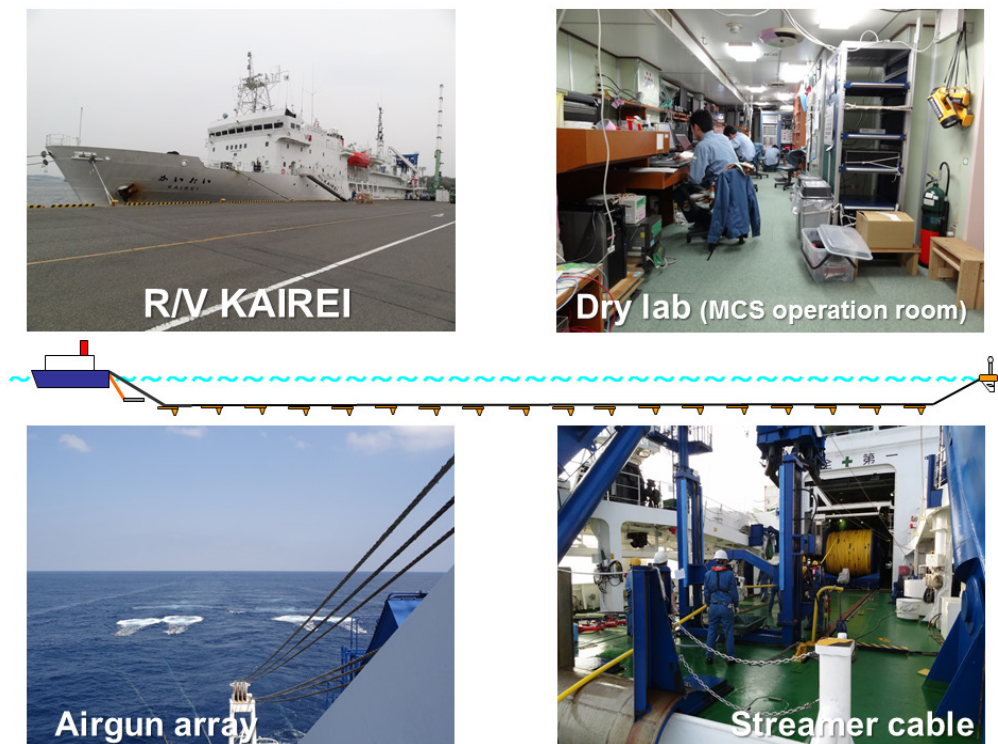
Fig. 2 MCS system on R/V KAIREI.
