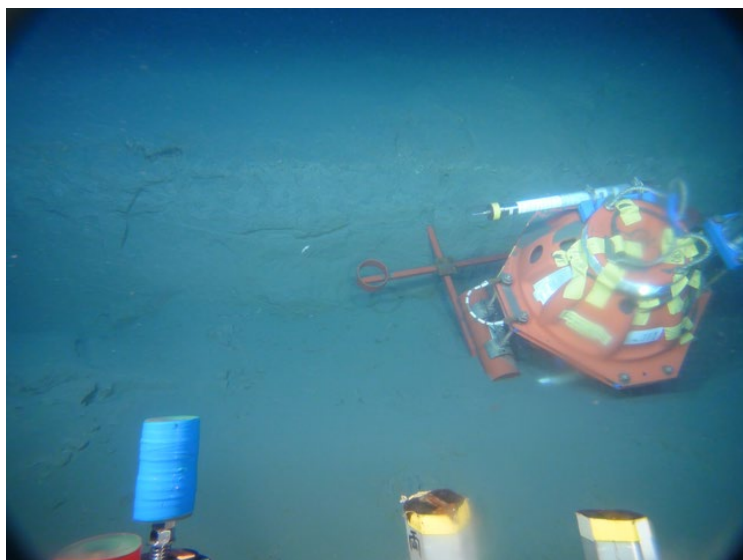
Fig. 5.4.2 Discovered a deep-sea OBS. A part of the anchor was buried in soft mud in a fissure.
