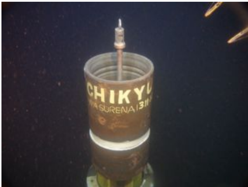
Figure 5.3.2 Wellhead of Hole C0019D and ROV hook eye.
