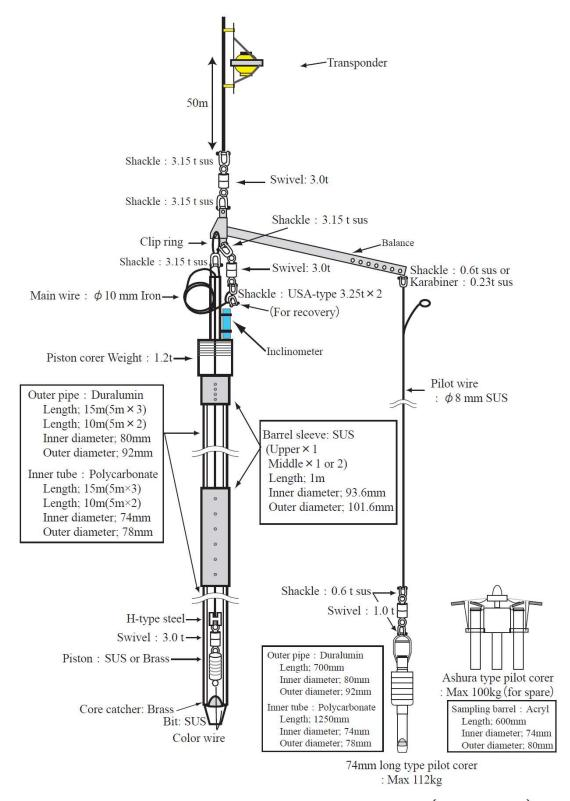
Construction of 10 or 15m PistonCorer (KR14-02)
