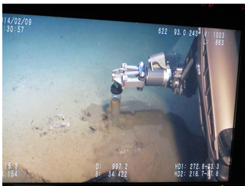
Figure 4 Sampling operation test by MBARI-type core sampler
