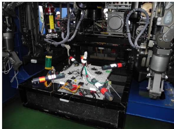
Figure 7: Receiver unit of TDEM system
