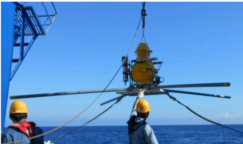
Fig. 3b OBEM of one-sphere type recovered at NM02 in the present cruise. The photo was taken at the deployment during the KR12-14 cruise.
