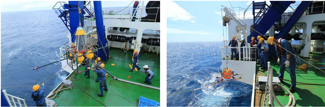
Figure 2: Photographs of the SFEMS using A-frame crane (left) and the LTOBS using davit crane (right) launching on the deck.
