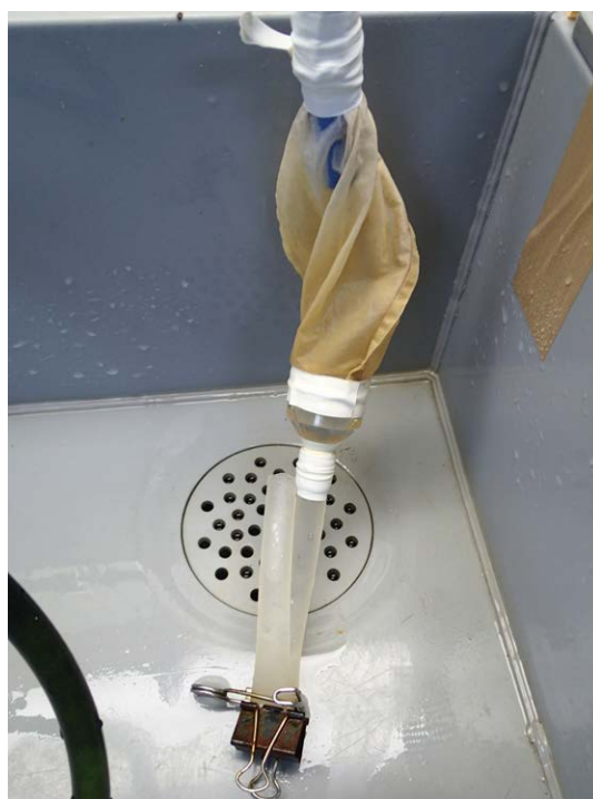
Figure 4.8 Plankton sampling system using pumped seawater.
