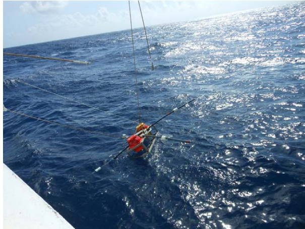
Photo 1. The OBEM recovered with the first long-term data at the site NM03.
