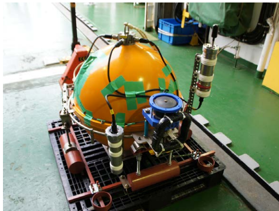
Photo 5. The rear view of the OBAT. The absolute pressure gauge (left) and the electro-magnetic current profiler (right) are equipped with the acceleration / tilt sensor on the leveling unit inside of the Ti sphere.
