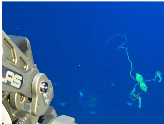
Photo 3. The floating rope of the OBEM imploded near the EFOS.
