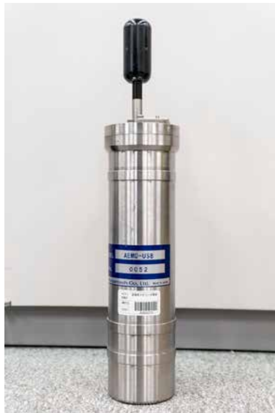
Fig.4.1.1. JFE Advantech AEMD-USB electromagnetic current meter, \phi 8.5 cm, height 42.1 cm. A biaxial electromagnetic field-induced sensor is installed at the top (painted by black rubber)
