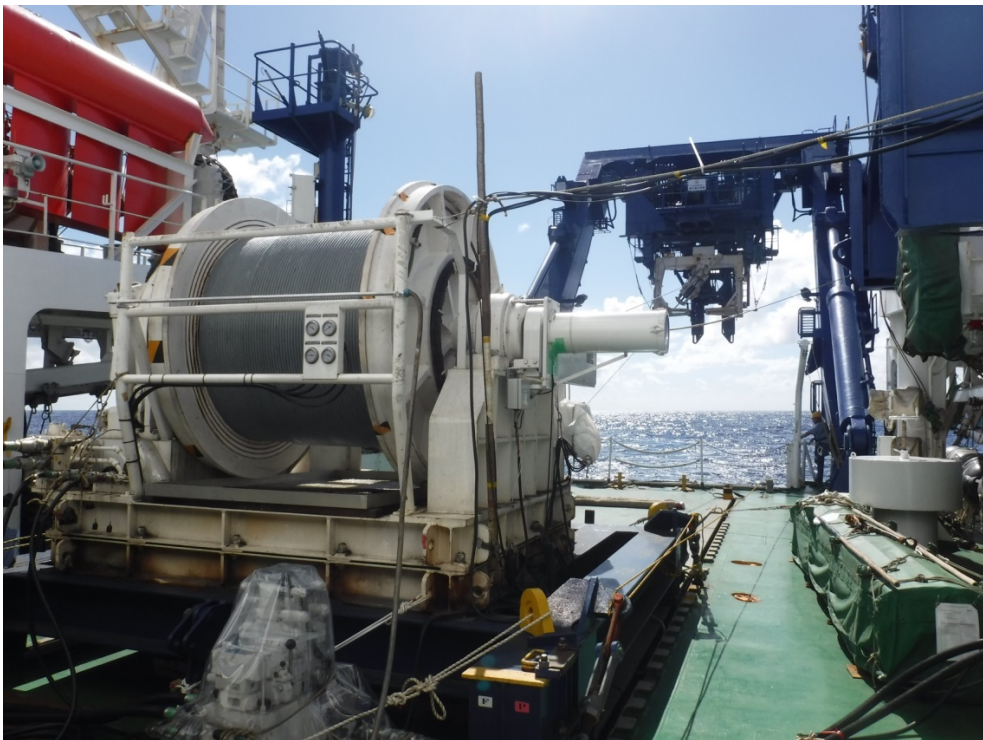
Figure 6.3: Optical-electric composite umbilical cable winch (No.15 winch).
