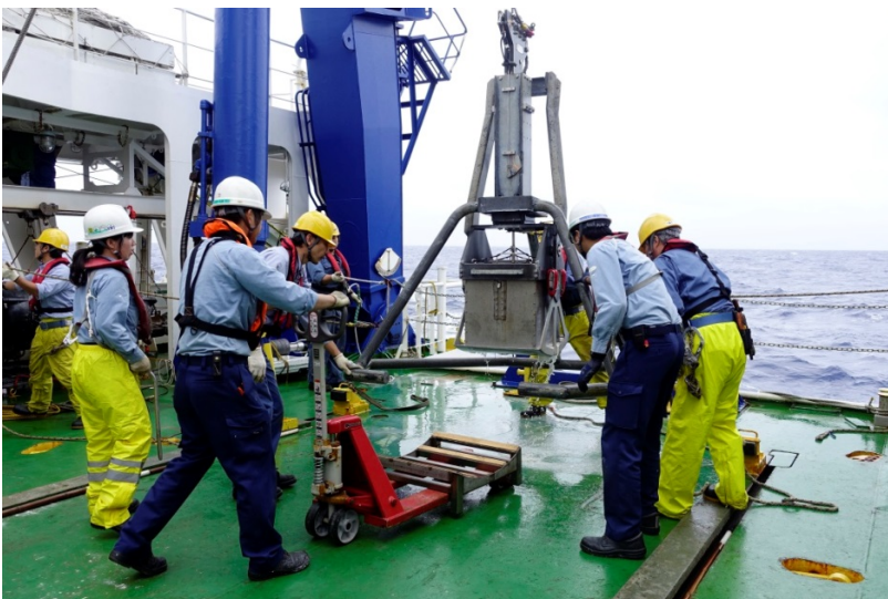
Figure 6.8: Box corer recovered. The spade has closed the bottom of the box and is supporting the sediment sample inside.
