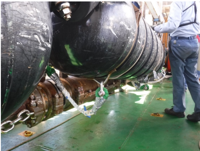
Figure 6.9: APG airgun in HR-MCS mode. Short depth adjustment ropes (1.5 m) were used.
