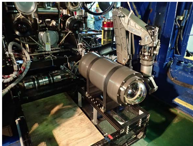
Fig. 3.4-1 USHV Camera blimp on KAIKO Mk-IV payload
