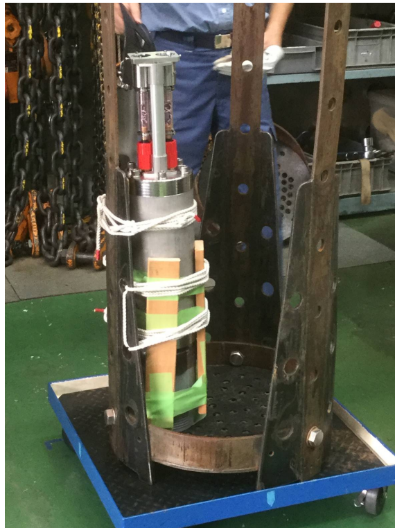
Fig. 3-5 Hydrothermal flow rate measurement apparatus using ultrasonic waves.
