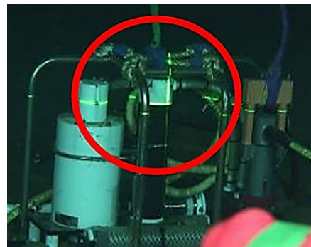
(b) Laser projected on DONET water pressure gauge
