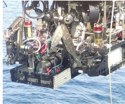
(b) Mobile pressure calibrator on basket for payload
