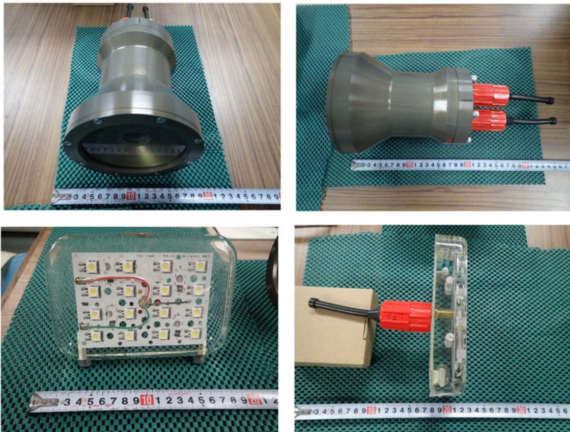
Figure 17. Deep-sea camera and light, which are attached to the Box Corer. Sony HDR-AZ1 video camera is in the pressure container of the deep-sea camera that can stand up to the pressure of 7,000 m water depth.
