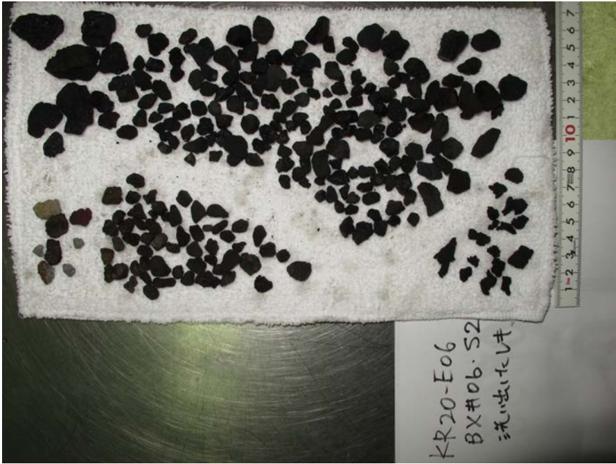
Figure 37. Recovered scorias, some of which have irregular elongated shapes. Most scorias are dark-colored without light-colored pumices.
