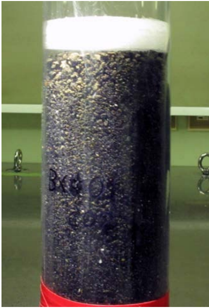
Figure 23. (Left) recovered sediment (~19 cm). (Right) a few mm of pumice are contained in addition to scorias and lava fragments.
