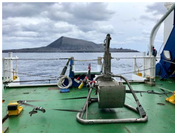
Figure 16. Box Corer. Size: 120cm (width) × 130cm (length) × 150cm (height). Weight: 260 kg The bottom of the box covers and samples an area of 0.1 m 2 (33 cm×33 cm) of the sea floor.
