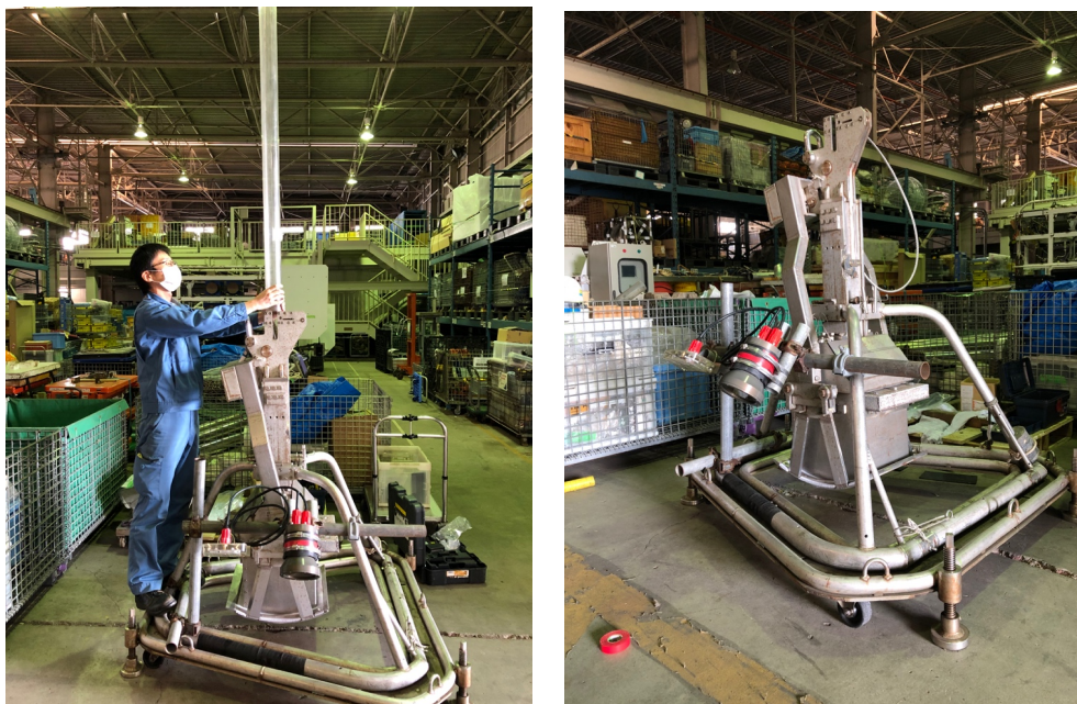
Figure 18. The deep-sea camera and light are attached to the box corer. The wire from the box corer is passed along plastic tube to prevent the wire from twinning around the camera and light.
