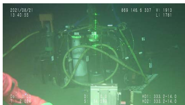
Fig. 3-4.2 DONET pressure gage during calibration
