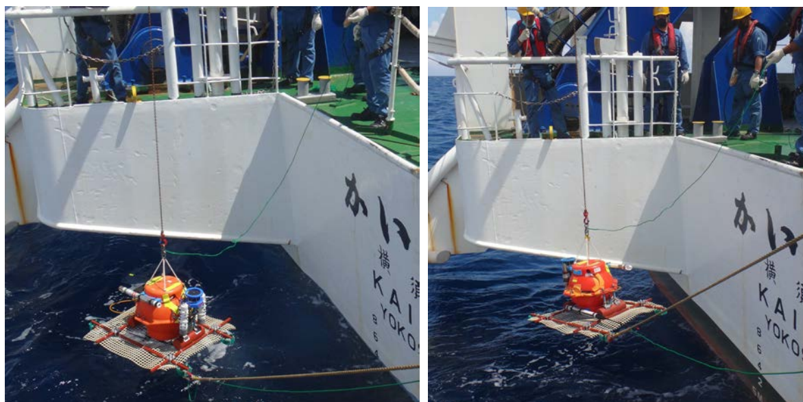
Fig3-2.2 Release operations of OBP(Left) and IES (Right)
