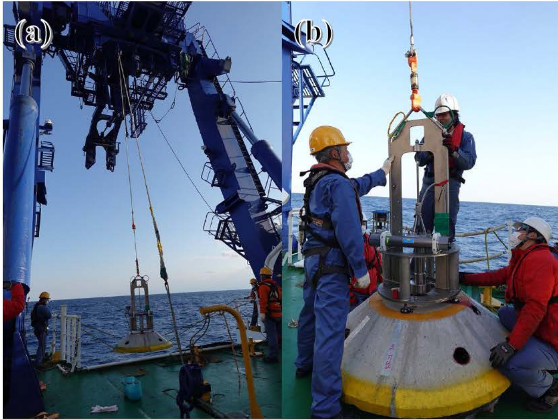
Fig. 6-2-3-2: (a) Cable connection of the CP release system. (b) Acoustic release system.
