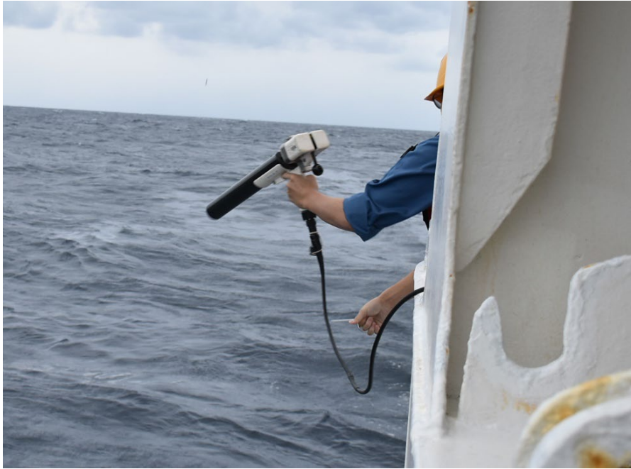
Fig.5-4-1: Release of XBT probe using XBT Launcher
