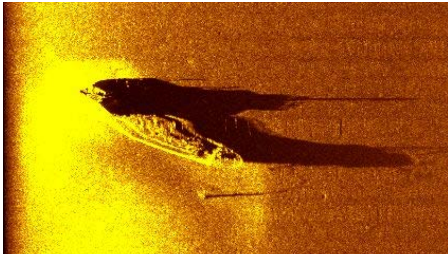
Fig. 3.7.8 Raw backscatter data obtained side scan sonar in this cruise.
