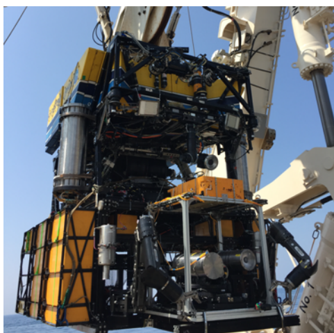
Fig.5-1 Mobile Pressure Calibrator on the sample basket of the HPD
