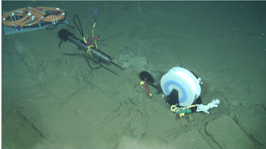
Fig. 3-3.1 Optical strain meter on the laying device
