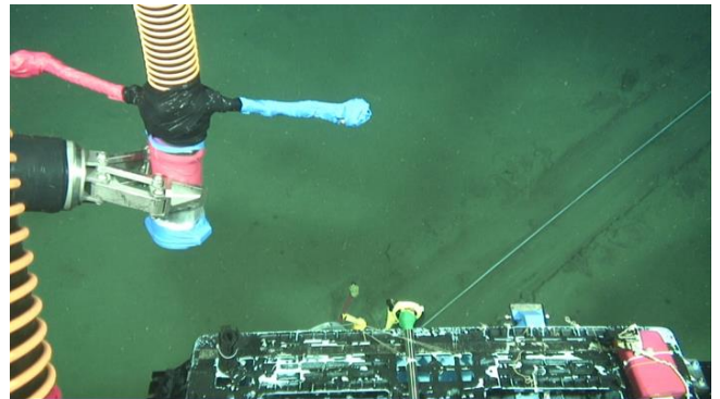
Fig.3-4.4 Strain meter laid on seabed
