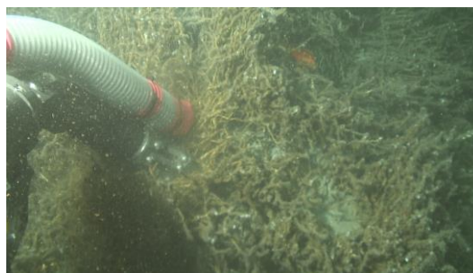
Collecting bio samples from the bush of tube worms using Vacuum water sampler
