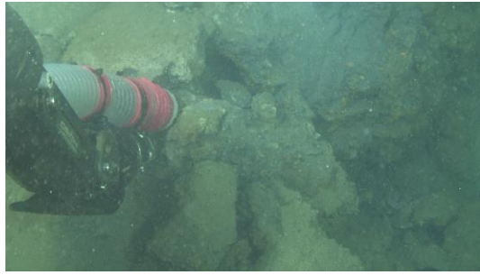
Sediment sampling with suction sampler
