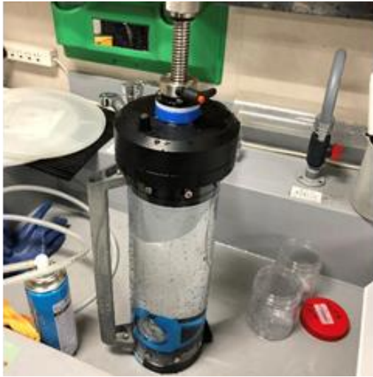
Fig. 1 The handy pressure vessel(left) and the eggs of L. satsuma in the sealed pressure vessel(right).
