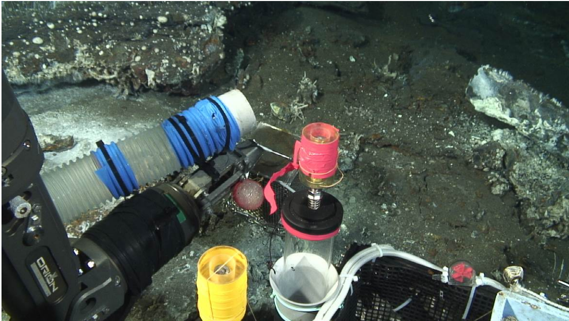
Fig. 3-38 Installation of the gold adsorption apparatus on the hydrothermal shimmering from cracks of seafloor rocks.
