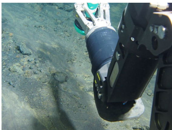
Sampling sediment using a push-core at 15:17:21
