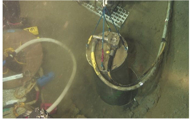
Photo 3. 1-2 Pull out the ground motion sensing system
