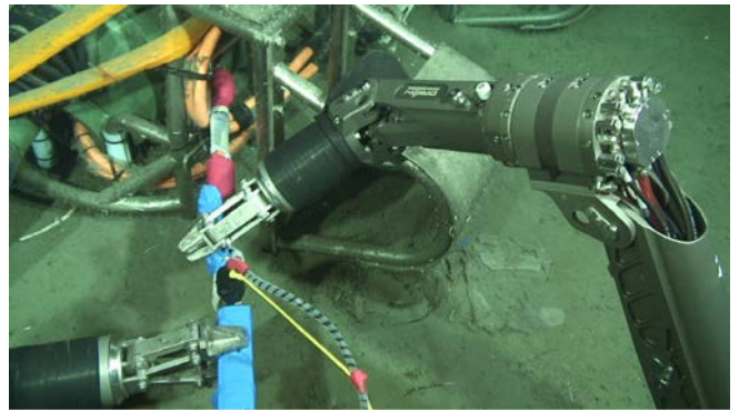
Photo 3.1-2 Checking the bulkhead connector.
