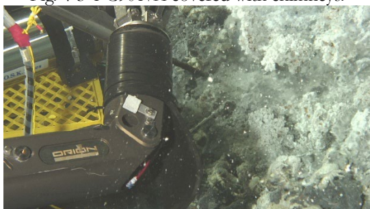
Fig. 4-4-1 Temperature measurement at the foot of Yubikuwae Chimney.
